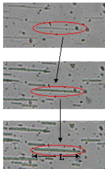
Fig. 6. An example shows how to calculate the maximum length of fibrous crystal.
